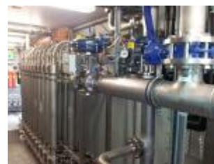
FIGURE 1: Biogas upgrading plants using highly selective membranes.
